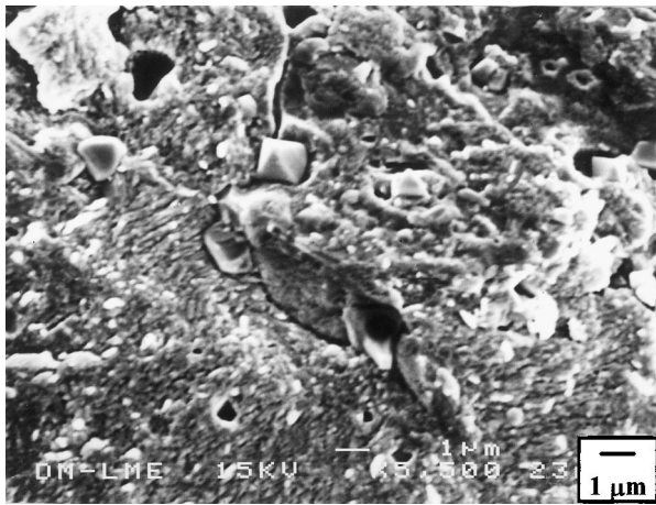
Fig. 9. SEM micrograph showing transgranular fracture and exposed spinel particles under stable crack propagation in (Mg,Y)-PSZ.
