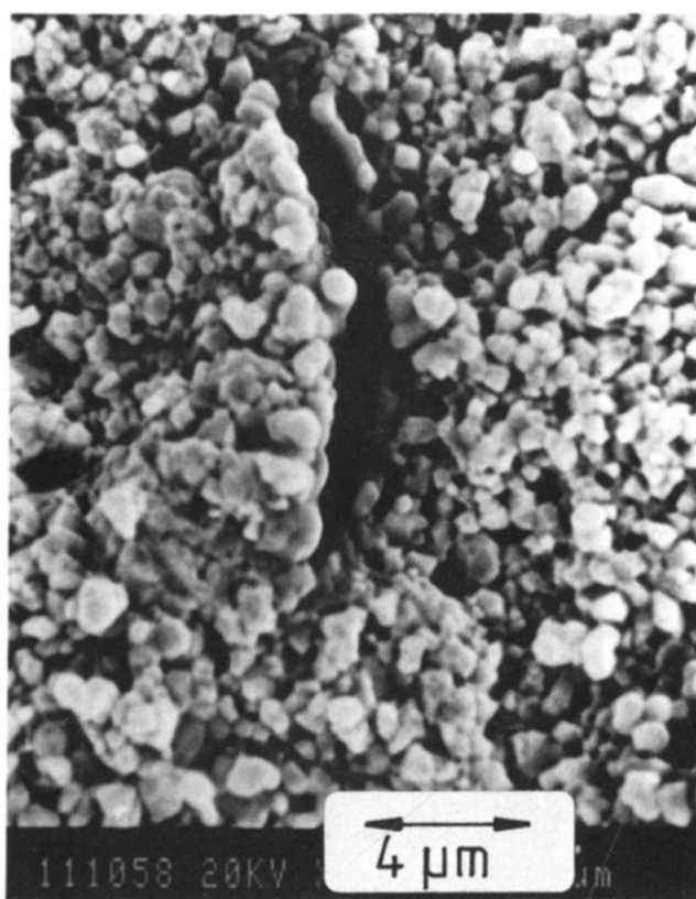
Fig. 11. Scanning electron micrograph showing fracture particle ZM15 (1400°C, 1 h).
